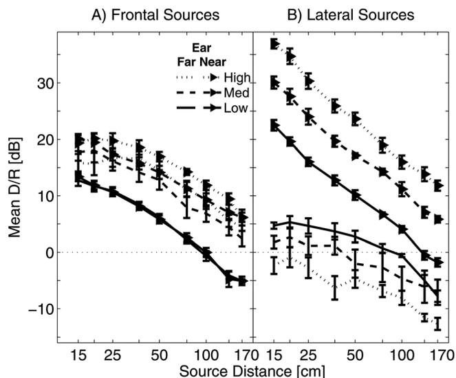
FIG. 3. Mean D/Rs for the narrowband stimuli used in this study, plotted separately for the far (left) and near (right) ears as a function of source distance. Across-subject averages ( $\pm$  SEM) in the measured D/Rs (averaged across the ten noise tokens) are plotted for each combination of stimulus spectral condition (line style) and direction [panel (A) vs (B)].
