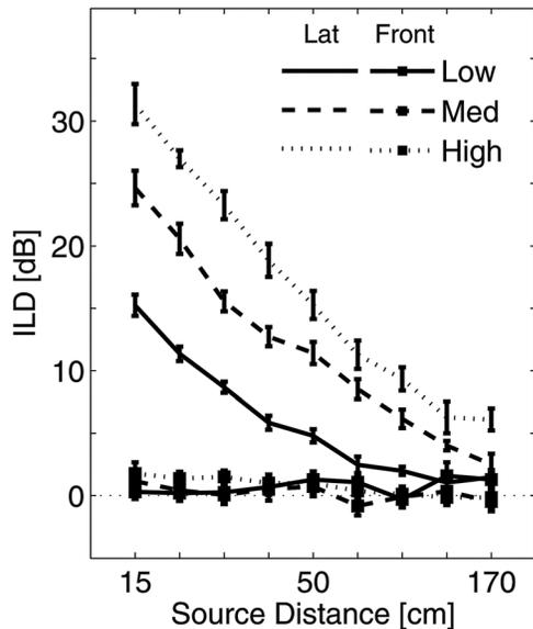
FIG. 4. Mean ILD for the narrowband stimuli as a function of source distance. Across-subject averages ( $\pm$  SEM) of the measured ILDs (averaged across the ten noise tokens used in each condition) are plotted separately for each combination of stimulus spectral condition and direction.
