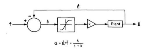
Proceeding from the left, eye velocity ( $\dot{E}$ , the time derivative of E, eye position) is subtracted from the target velocity ( $\dot{T}$ , the time derivative of Target position, T) to yield retinal slip (target-fovea offset) velocity ( $\dot{e}$ , the time derivative of slip, e). This signal is passed through a saturating nonlinearity, depicted by the box containing a sigmoid curve.
